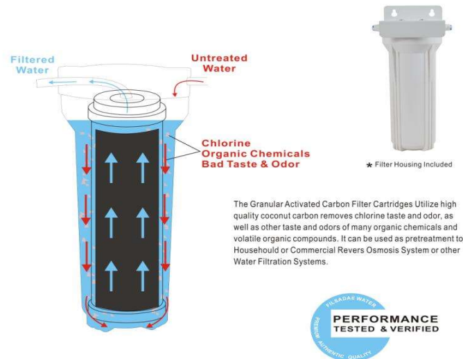
Figure 36: Overview of Filtration process in water filter
