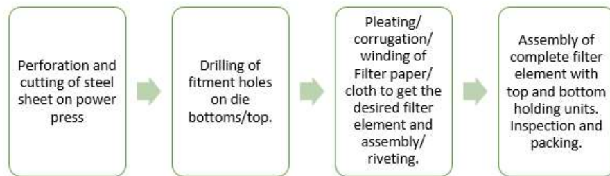
Figure 33: Manufacturing process of air filter
